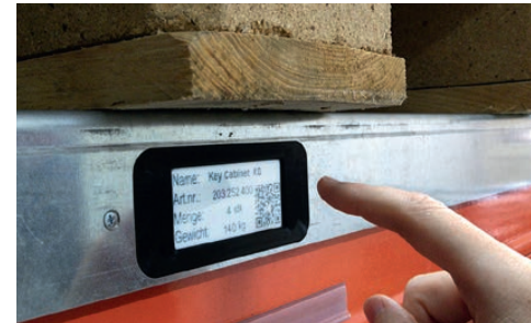
ESL signage on each pallet location
