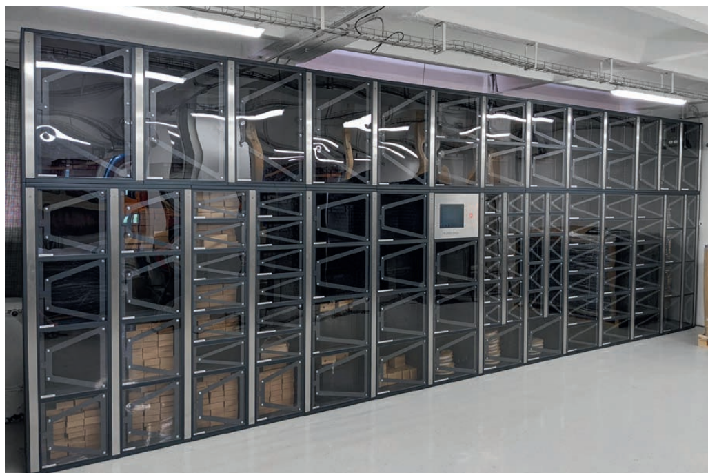
system with special height up to 250cm for management of raw products and produced semi-finished products
